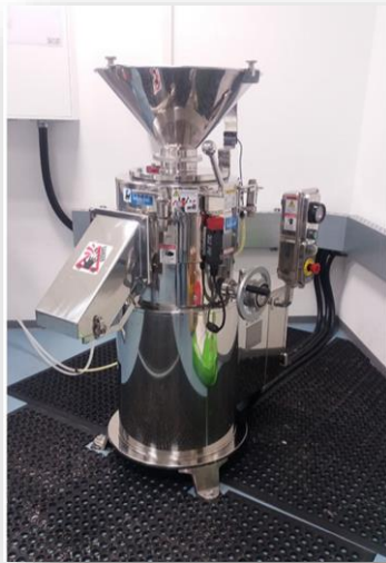
Grinder of Pilot Line 10
