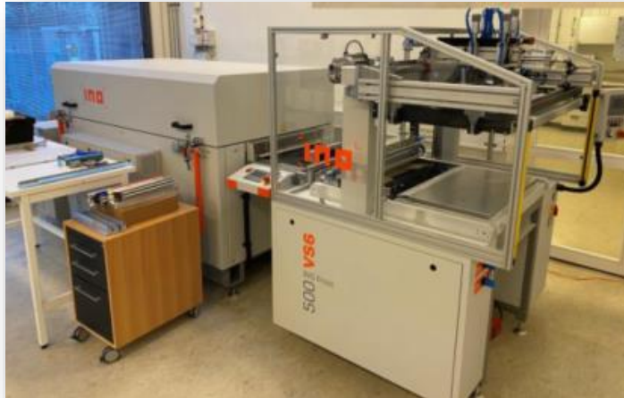
Screen printing facilities of Pilot Line 16
