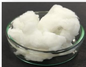
Commercial eucalyptus pulp processed to obtain nano-cellulose
