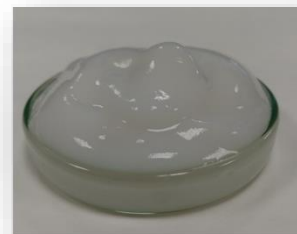
Commercial eucalyptus pulp processed to obtain nano-cellulose
